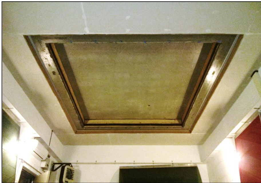
Receive Room View of Test Specimen Installation
