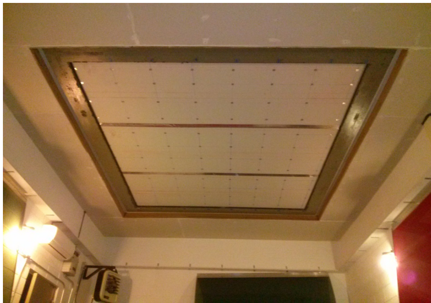
Receive Room View of Test Specimen Installation
