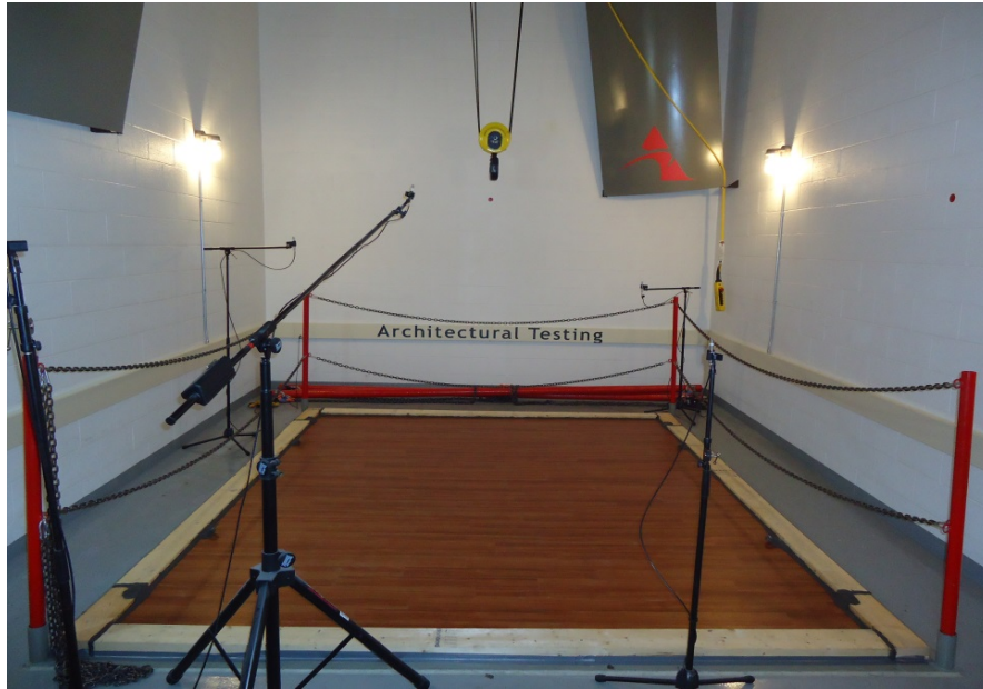
Source Room View of Test Specimen Installation
