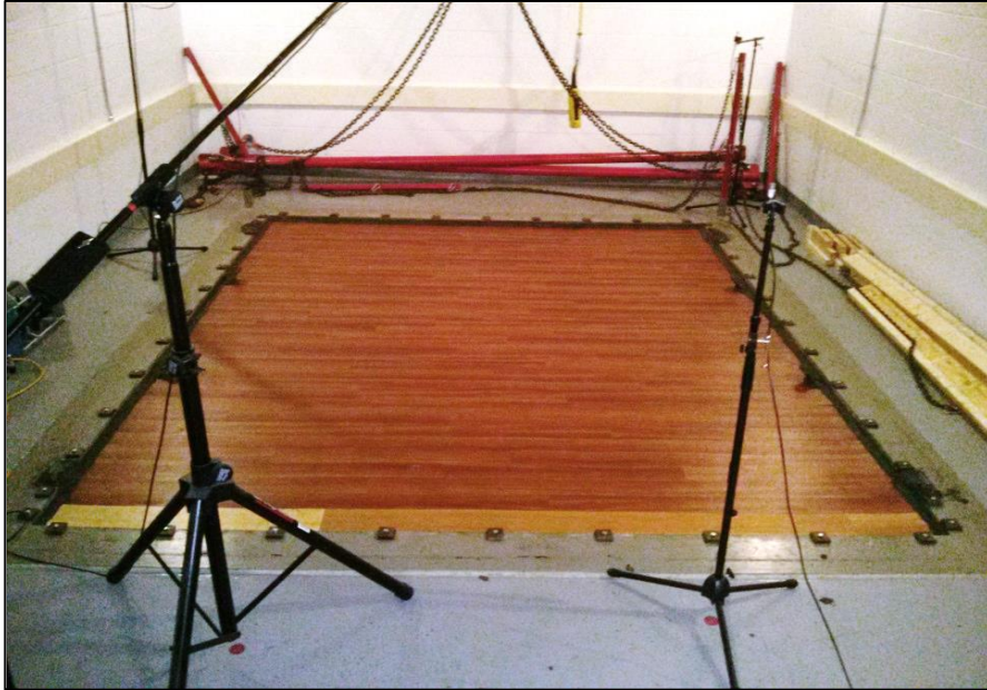
Source Room View of Test Specimen Installation
