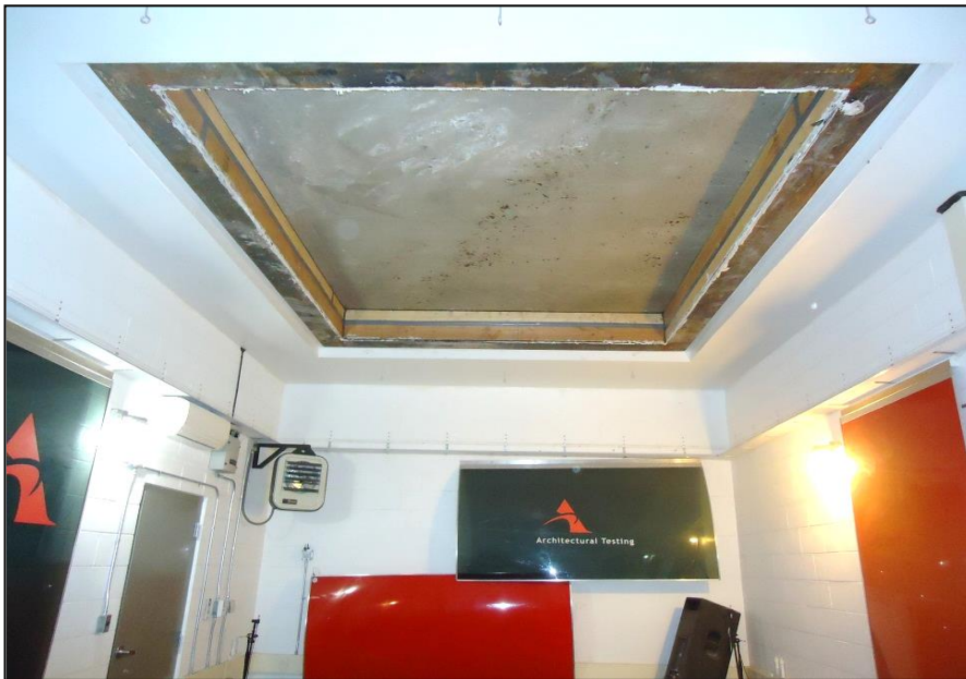
Receive Room View of Test Specimen Installation
